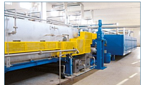
Horizontal steamer, washing unit and dryer
