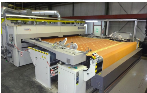
Stenter inlet to dryer
