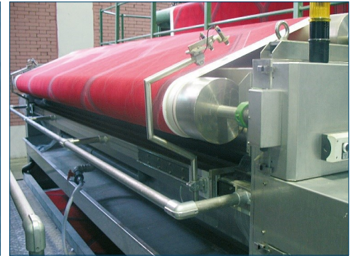
Foam application and impregnation
